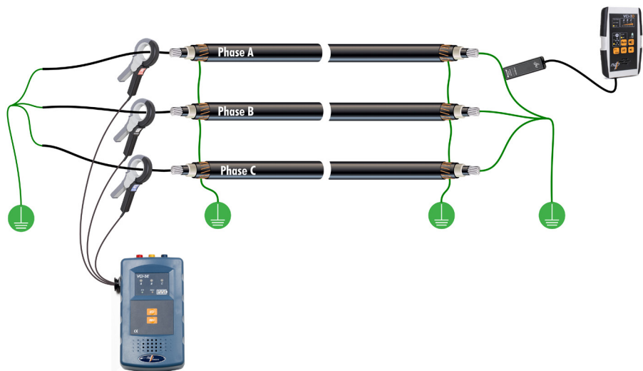
Typical cable identification setup
