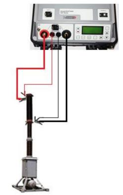
GGT500 cable connection on live-tank circuit breaker
