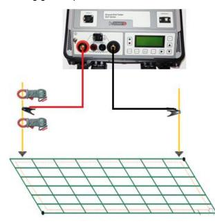
GGT500 cable connection for ground grid test
