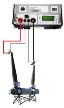
GGT500 cable connection on dead-tank circuit breaker
