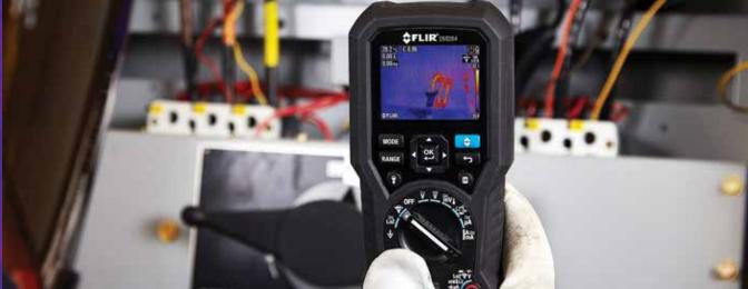
Troubleshoot easier with the unique combination of onboard thermal imaging and traditional Digital Multimeter test functions.
