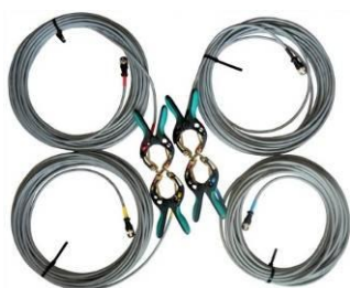
H winding test cable set
